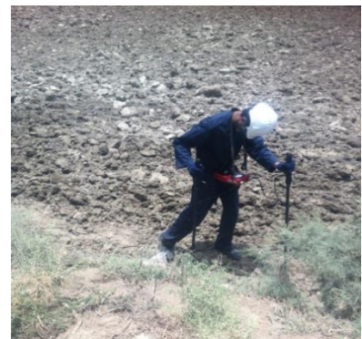
Oilman staff carrying out DCVG Survey at a pipeline in interior Sindh
